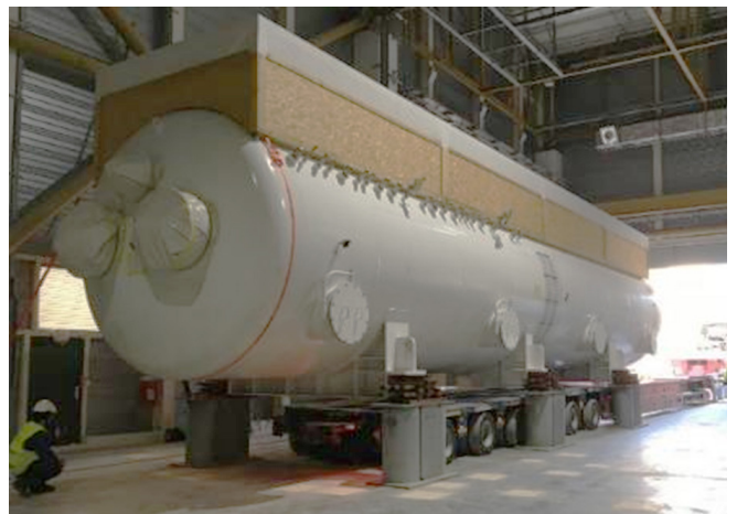
Figure B.4 Cryoplant Termination Cold Box (CTCB) transportation to the ITER site
