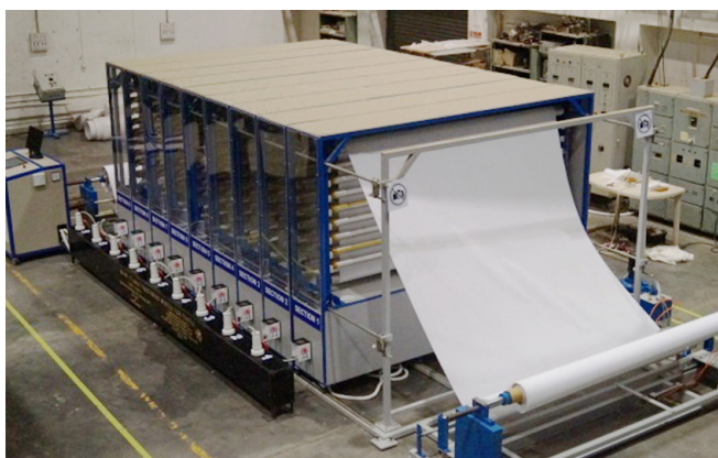
Figure A.1.3 A photograph of the inline textile treatment facility
