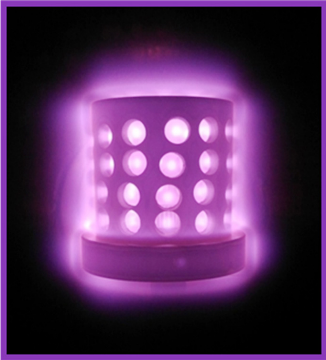
Figure A.2.1 Active screen plasma nitriding
