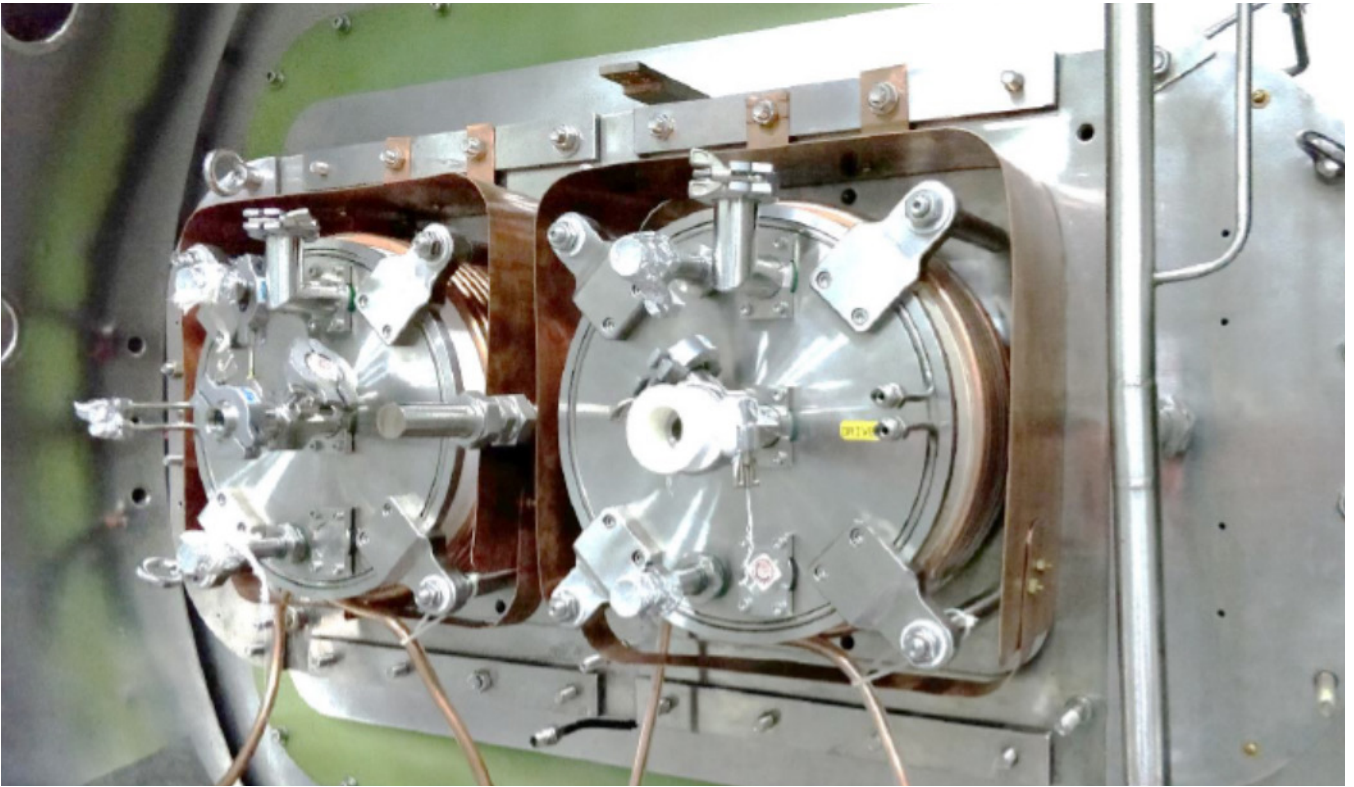
Figure A.4.3 Two driver RF based negative ion source - Twin Source operational in IPR
